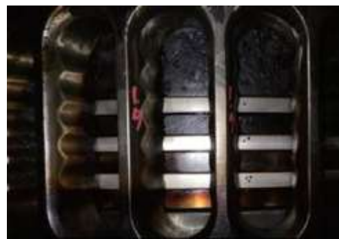
Photo 2 Medium amount of deposits on 1 st ring land (Quote: MAN Energy Solutions, Service Letter SL2019-671)
